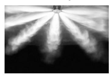
Low heat of vapourisation 95 kJ/kg Vapour pressure 40.4 kPa Super-pressurised with N2 Nozzle design
