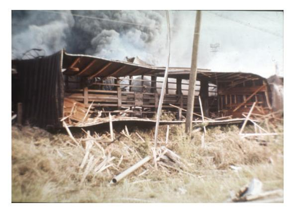
The explosion under these empty truck transport tankers caused one to completely flip over and the next one, which was only  $\frac{1}{2}$  over the vapor cloud, to flip up in the air and lean on the next trailer. The third trailer, which was almost completely outside the vapor cloud, was only dented in on the front of the tanker but the truck was totally destroyed. The vapor cloud was from a gasoline tank overfill.
