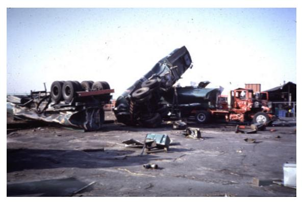
In another gasoline tank overfill, the pickup below had the front  $\frac{1}{2}$  over an explosive overpressure but the back portion was not. The front  $\frac{1}{2}$  of the truck is missing the fenders, hood, and cab. Note you can see through the frame to the pipes on the other side. The rear of the pickup bed is only burned by the ensuing fire and not distorted by an overpressure. The truck was flipped over on to the pipe rack by the explosion under the front of it.
