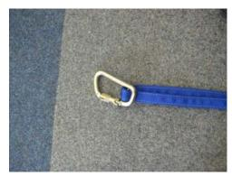
During pre-use inspection, if the web appears to be threaded around the pin, then the lanyard should not be used.
