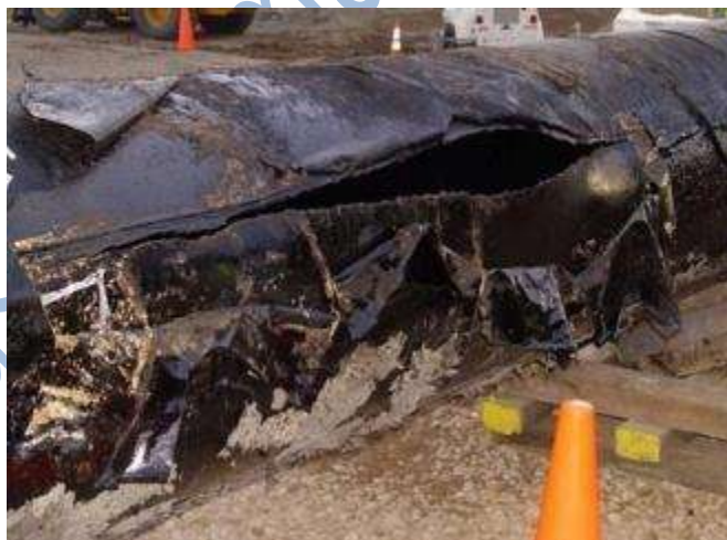
Section of pipe containing rupture. Rupture length is approx 6 ft 5 inches and is 4 1/2 inches wide at the widest location.
