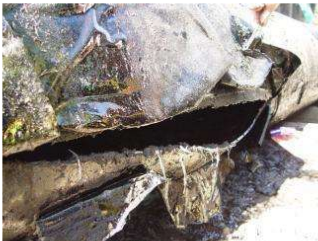
Close-up view of the section of pipe containing rupture. Rupture length is approx 6 ft 5 inches and is 4 1/2 inches wide at the widest location.
