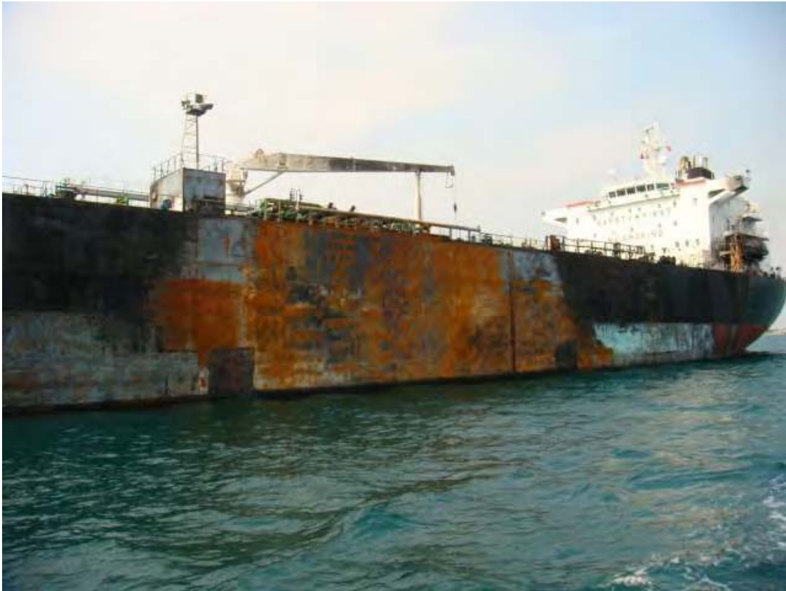
Damage to side shell of vessel
