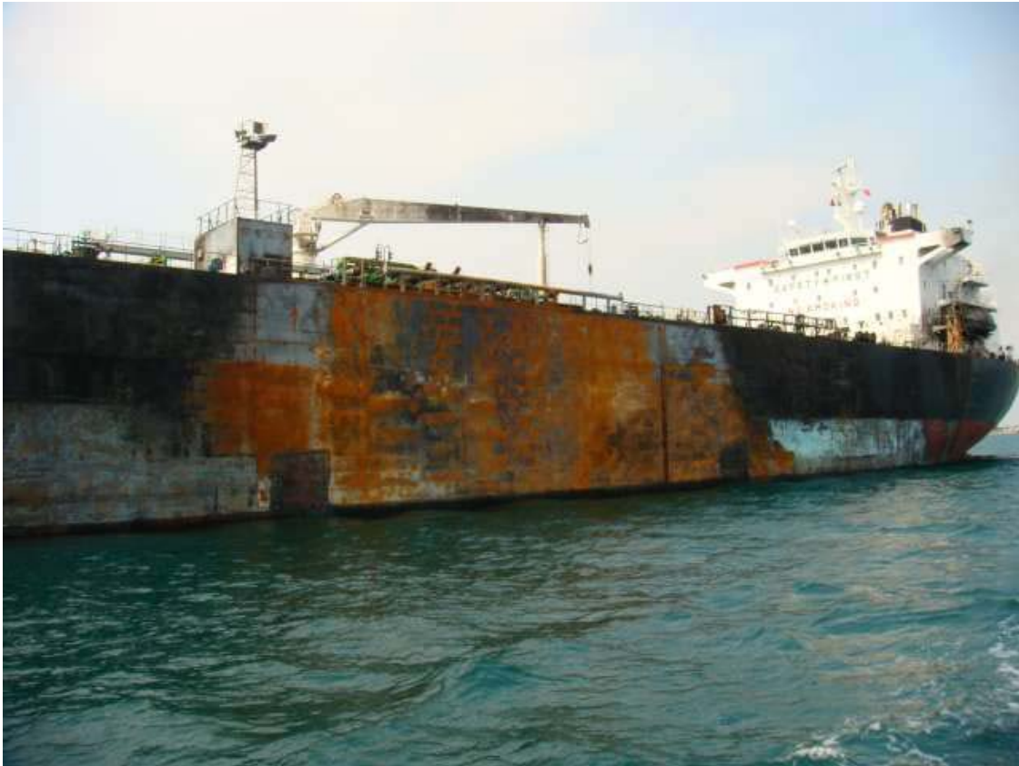
Damage to side shell of vessel
