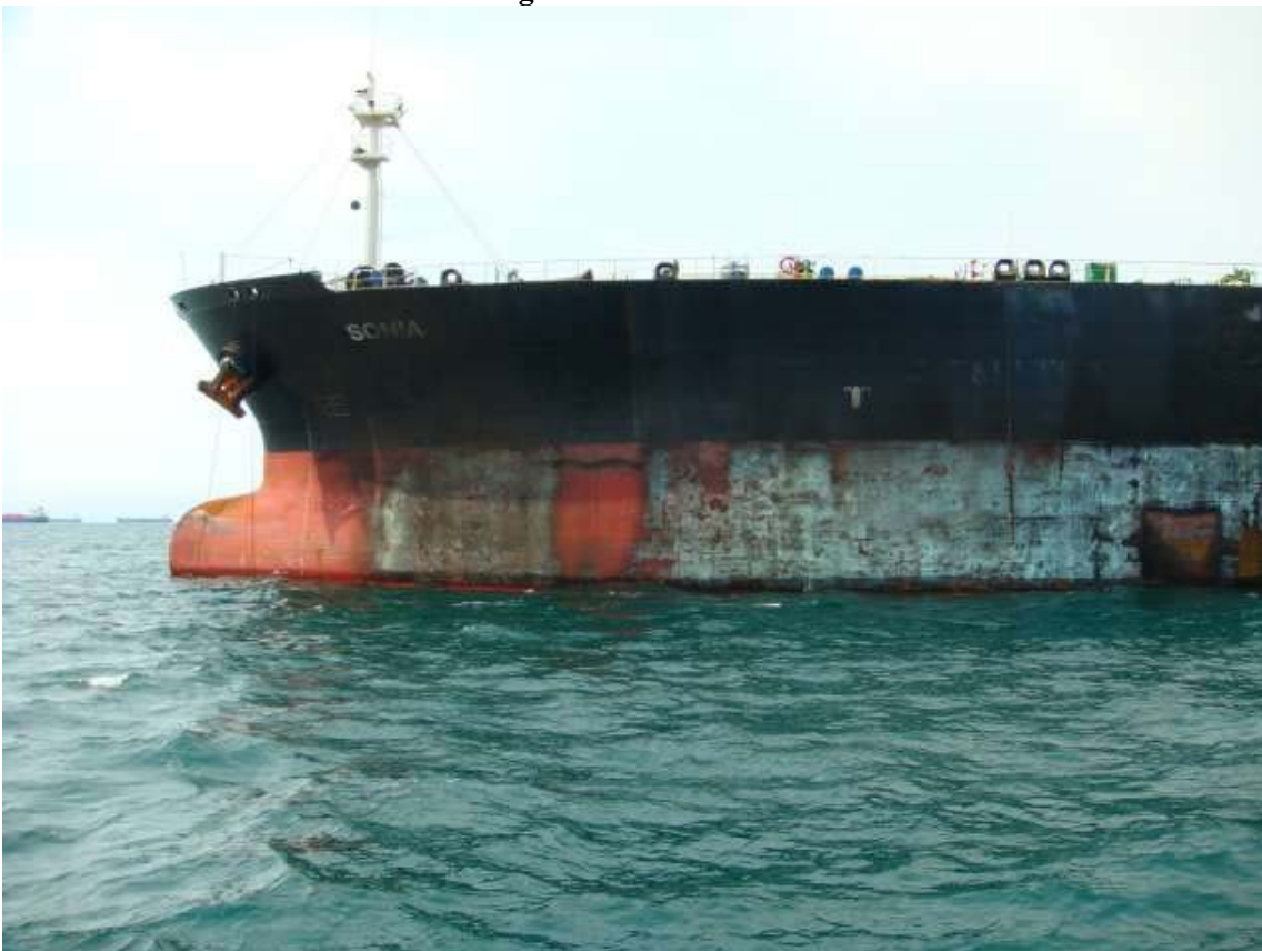
Damage to side shell of vessel
