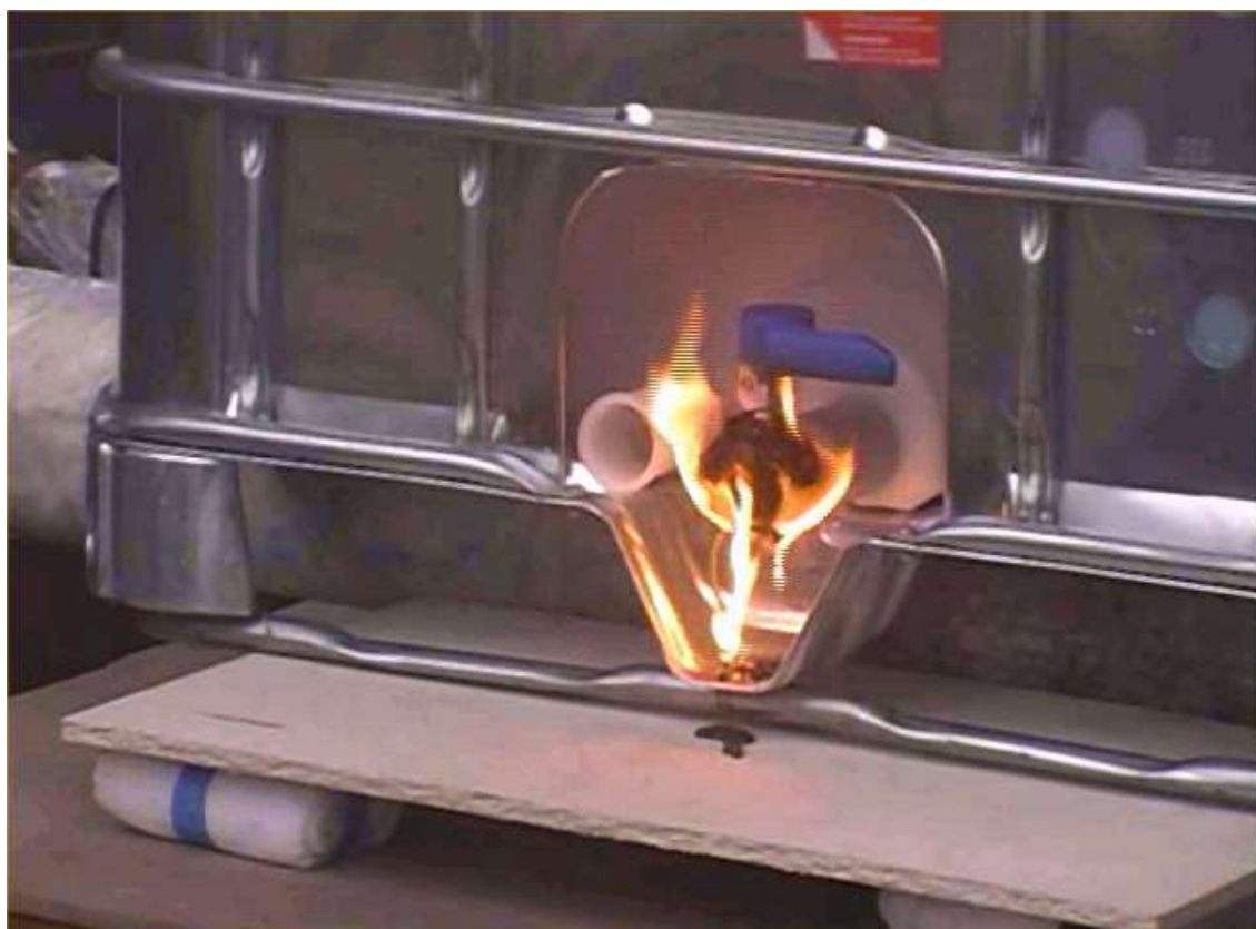
Figure 11: False floor on thermoplastic foam supports
