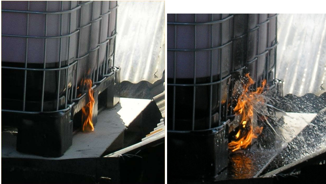
Figure 16: Small fire at the edge of the pallet of an IBC containing a mineral oil lubricant. Early failure occurs where flames impinge on the inner receptacle.
