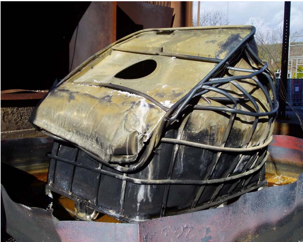
Figure 25: Crushing of lower (water filled) IBC by an upper IBC loaded with bricks (970kg) during fire engulfment Above – extent of initial (arrested) yielding. Below - extent of damage following final uncontrolled collapse.
