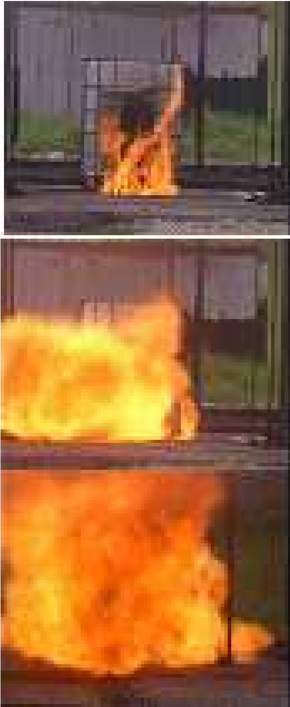
Figure 10: Consequences of ignition of IPA vapour in the ullage of a part-full IBC
