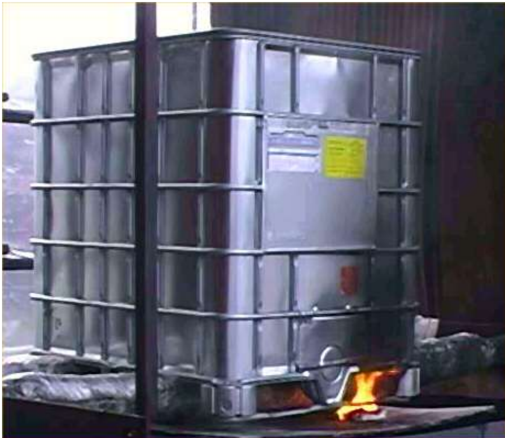
Figure 17: A small fire under of the pallet of a metal clad IBC containing a mineral oil lubricant. Failure of the base of the inner receptacle occurs even though this is protected by the folded metal sheet forming the top of the pallet.
