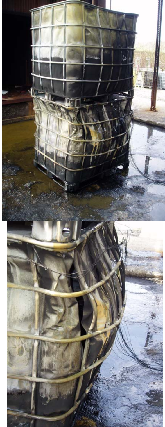
Figure 24: Damage to a stack of metal clad IBCs during fire engulfment. Separation of metal cladding sheets is visible in lower (closeup) view.
