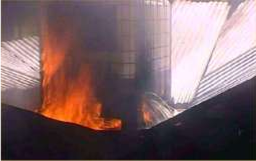
Figure 4: Inclined sheets used to capture spigot flow
