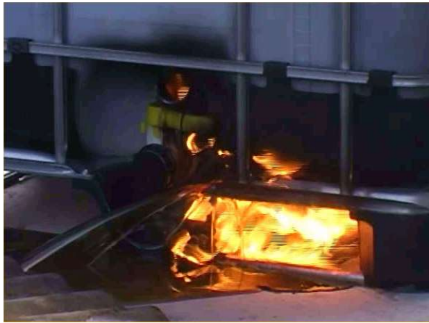
Figure 21: Fire in an IBC containing an industrial lubricant (flashpoint 196°C)
