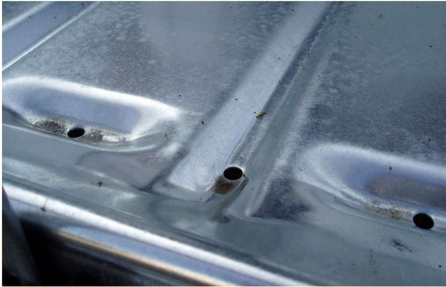
Figure 18: The top of a metal pallet – formed into folds to increase stiffness.
