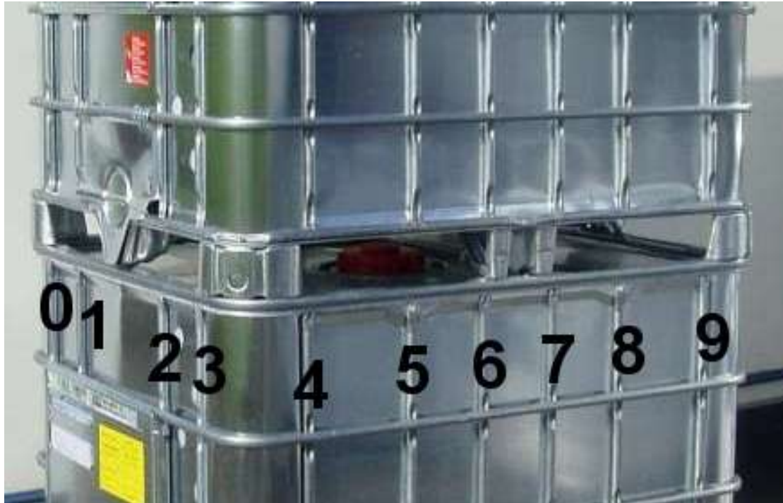
Figure 8: Locations of thermocouples recording steel tube temperature
