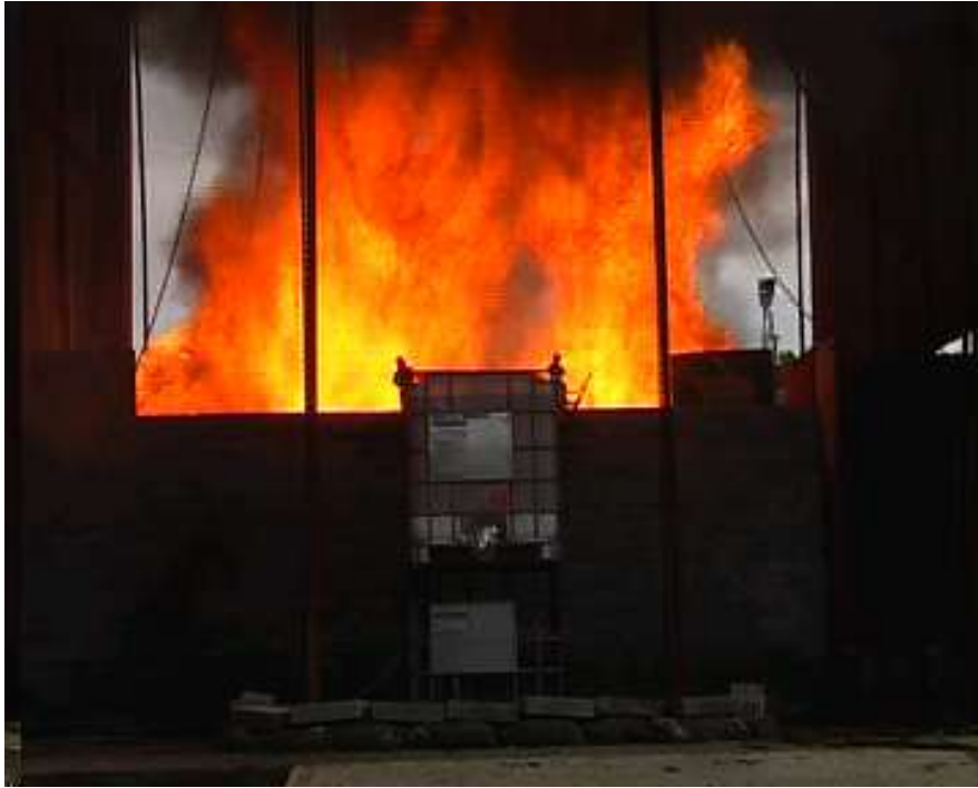
Figure 5: Typical view of flame shape relative to target IBC
