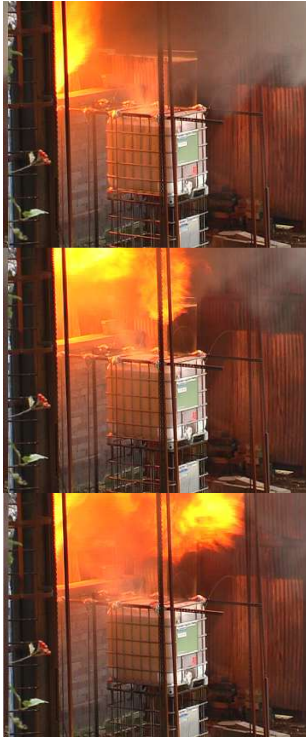
Figure 8: A sequence of images showing heptane combustion. This event was accompanied by a loud bang.
