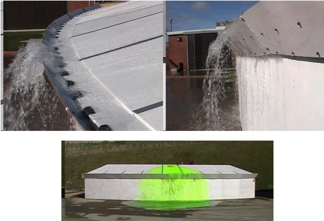
Figure 5 Photos of overflowing experiments from a section of a fixed roof tank showing liquid spilling over the deflector plate.
