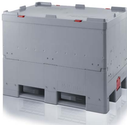
Image 6: Collapsible composite IBC with flexible inner receptacle, with composite butterfly or ball valve, with fitted composite pallet
