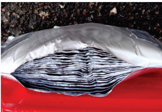
Figure 4 Ruptured lithium-ion pouch cell.
