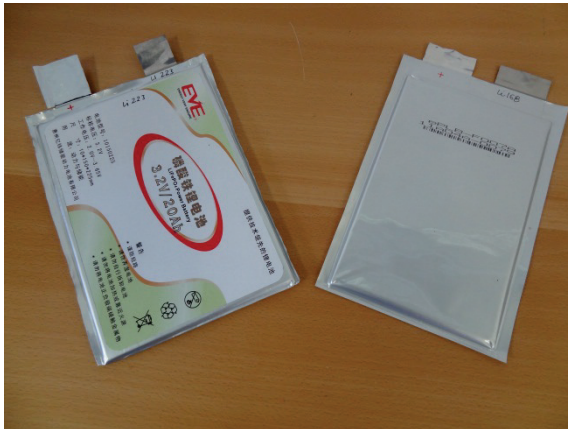
Figure 2 Two examples of lithium-ion pouch cells.
