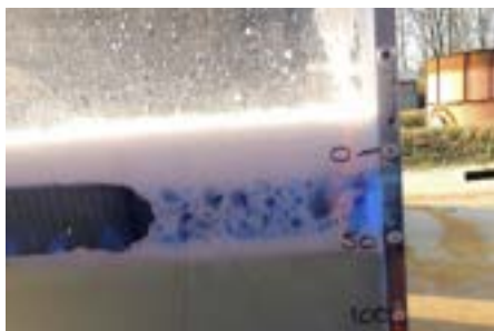
Figure 2. Side view of foam from a pourer plunging through 50mm of fuel. Note foam in the fuel.
