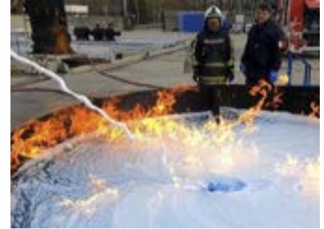
Figure 11. Discharge from Uni 86 Monitor nozzle with mesh - note "rope" of foam - and consequent heavy impact
