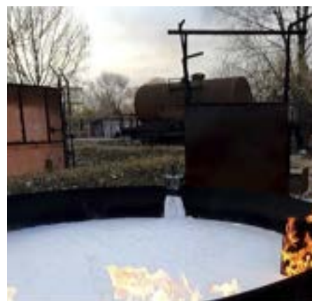
Figure 8. Foam pourer adapted to give gentler application - note impact point is extinguished
