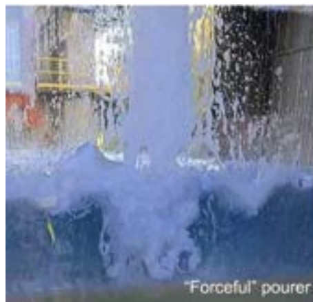
Figure 5. Comparison of plunging effect with different pourer arrangements into 100mm of fuel.
