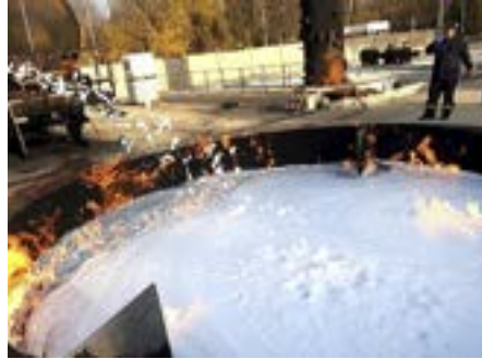
Figure 10. Discharge from standard (without mesh) Uni 86 monitor nozzle - note foam break up and consequent relatively gentle application
