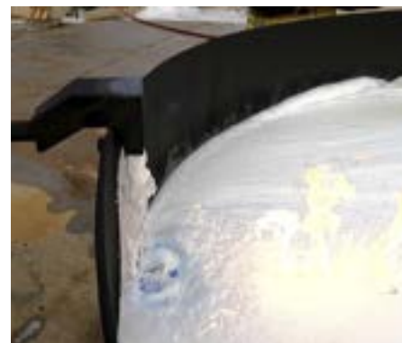
Figure 6. The forceful pourer clearly showing foam blanket exposure penetration and fuel exposure, with fuel pick up causing continuing burning on the foam surface in front of the impact point.
