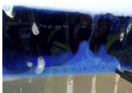
Figure 3. Photo of foam resting on interface of fuel and water
