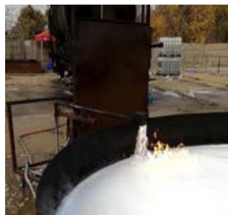
Figure 7. Another illustration of the impact point continuing to burn with the forceful pourer
