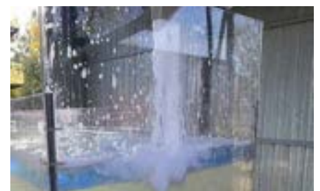
Figure 1. Foam from a "pourer" plunging through 50mm of Jet A fuel (coloured blue
