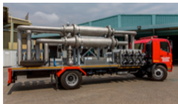
Sasol fire truck fitted with the ILS water filtration system
