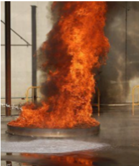
Image EN 1568 test. From http://www.fireengineering.com/articles/2016/02/environmental-influences-on-firefighting-foams-an-international-seminar.html
