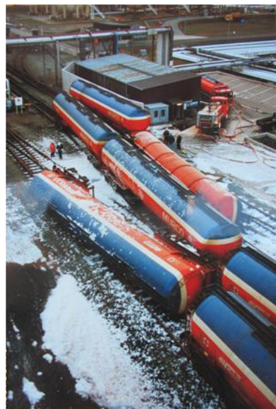
Derailed at rail loading bay, all tanks were full of petroleum spirit at the time
